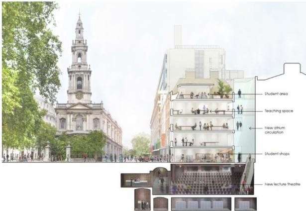
A drawing showing how the buildings will be used. A glass atrium at the rear accommodates the differing floor levels
